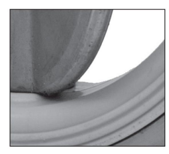
Accurate and smooth machined profile of disc edge requires minimal deformation of the resilient elastomer liner to achieve a positive seal. The low deformation results in low torque, less wear of the seat liner and increased operational life.
