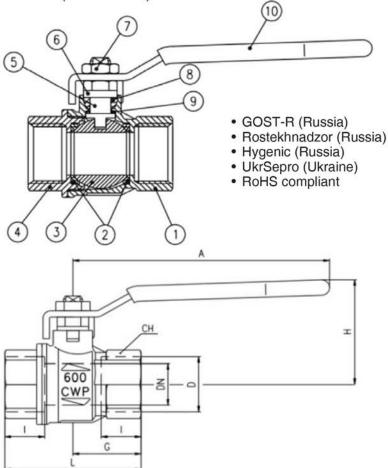
DN shows the nominal flow diameter. Actual flow diameter complies with full port DIN 3357 part 4. Stem configuration of valves over 2" is slightly different. Ask for details at our Service Center
