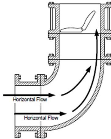
In this position, the valve rib is perpendicular to the incoming horizontal piping which creates an unequal loading on the plates.
