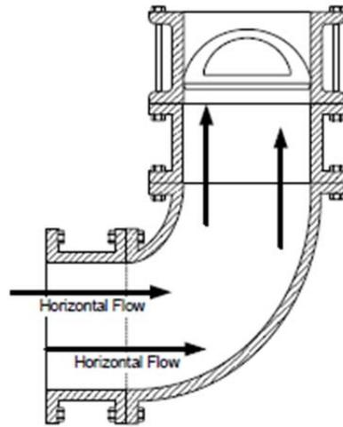
In this position, the valve rib is parallel to the incoming horizontal piping and creates an equal loading on the plates.
